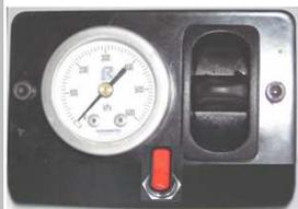
This is designed so that your air helper springs can be adjusted from inside the vehicle. A Dual cab control kit is suitable for controlling 2 airsprings independently and can tee them together by having the Left-Right air control in the centre
