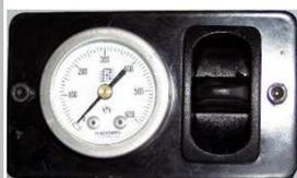
This is designed so that your air helper springs can be adjusted from inside the vehicle. A Single kit is suitable for controlling 2 airsprings Teed together, or otherwise one airspring. Moving the paddle switch upwards raises the vehicle, downwards lowers.
